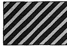
SKERPDRAAICHEVRON - LINKS SHARP CURVE CHEVRON - LEFT
