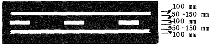
SPERSTREPE MET MIDDELSTREEP BARRIER LINES WITH CENTRE-LINE
